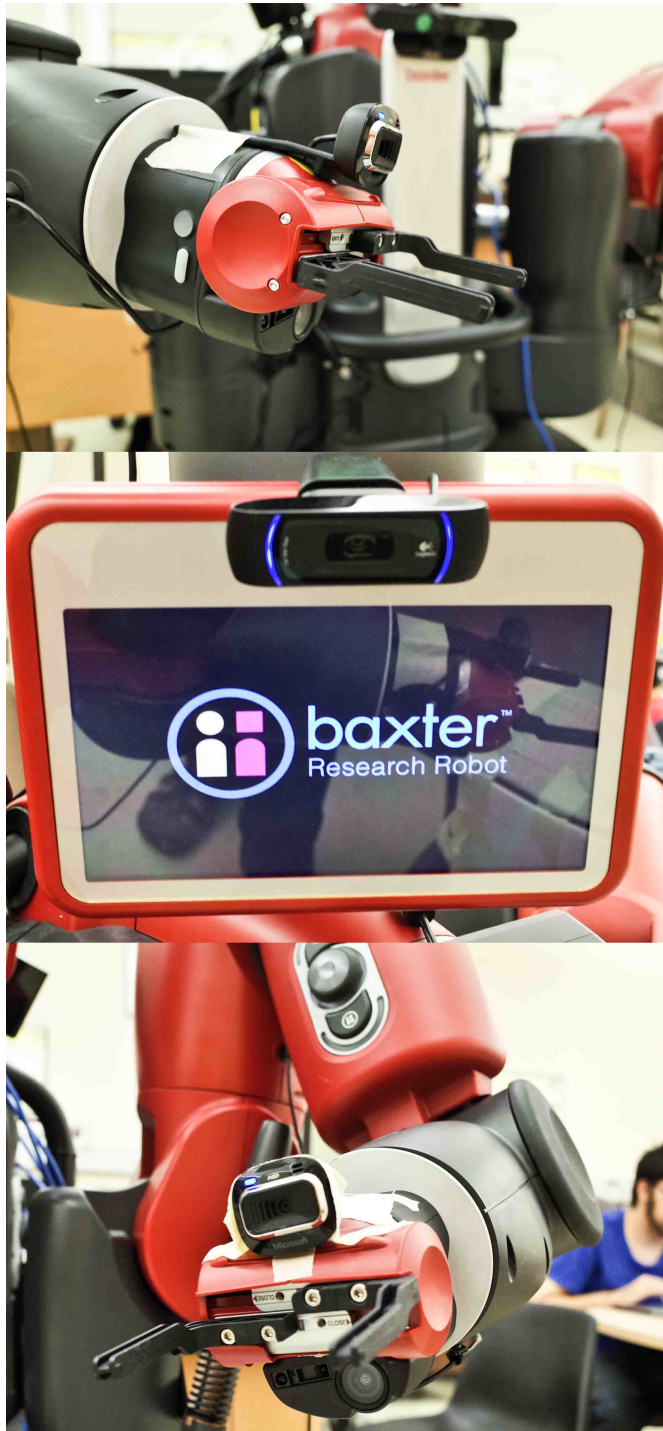
Figure 5.13: Webcams on Baxter's Right Arm (Top), Head (Middle), and Left Arm (Bottom).
