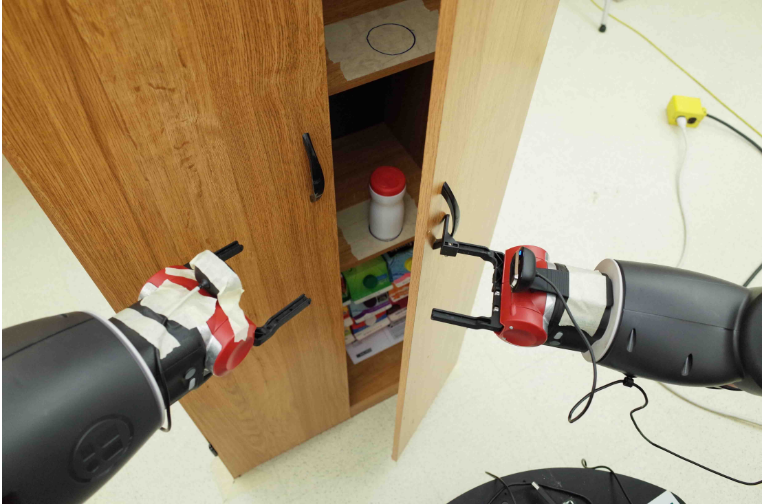
Figure 6.5: Baxter Is Opening the Door of a Cabinet.
